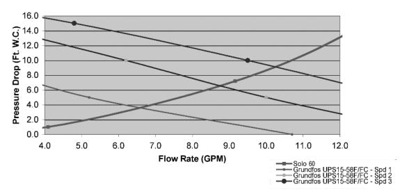
Note: Minimum allowable flow rate at full input: 3 gpm SOLO 60
